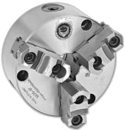
High quality cast iron body with precision machined guideways and bearing surfaces, drop forged case hardened scroll plate and hardened and ground pinions. 1 set of hardened reversible two piece jaws, 1 self ejecting wrench, 1 set of mounting screws, 2 allen keys and mounting plate provided.
