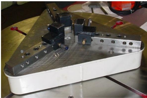
The Gripper is a cam operated assembly designed specifically for the welding industry. The gripper incorporates many features that make it especially suitable for the welding environment. These features include single point cam operation of the jaws and adjustable quick-change reversible jaws that can be positioned for small and large diameter work pieces. Heavy-duty construction and a completely enclosed faceplate prevents flux and weld splatter from impairing the operation of the gripper.
